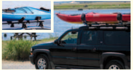
Right-side up using a Hullavator, inset using saddles
