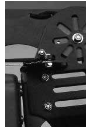
Close up of bushing, roller guide, and control cables.
